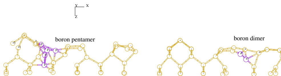
Figure 4. Interstitial boron clusters on SBN. The locations of boron atoms are indicated by the darker dots. The impurities are the boron pentamer and dimer whose atoms are labelled p and d, respectively. s and s1 indicate second-layer silicon atoms interacting with the boron clusters.
